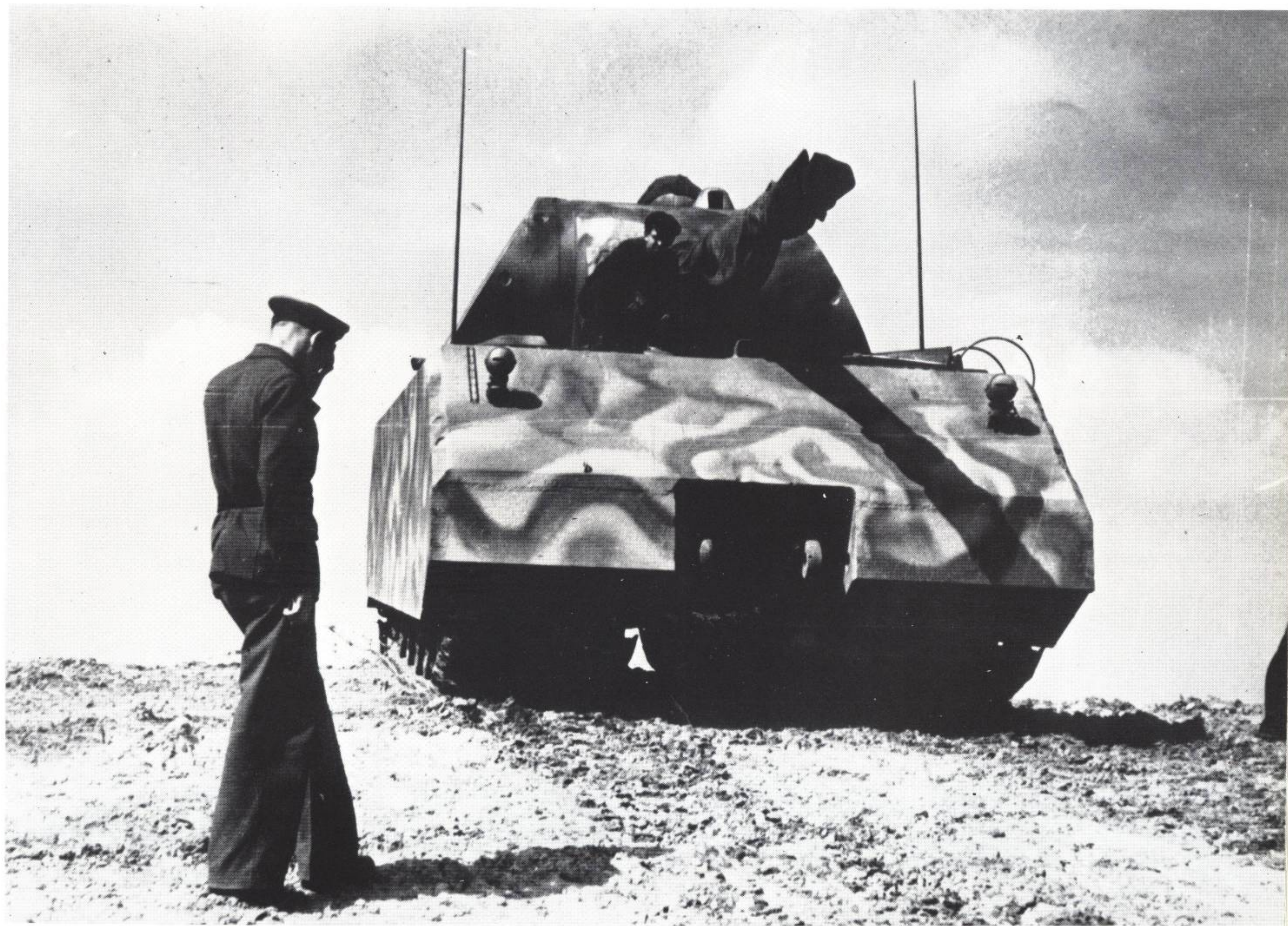
An imposing front view of the Maus, showing the two antenna masts. Aiming the cannon was done with the help of an elevation gauge, aiming telescope and elevating machine operated by the gunner. The arc of elevation ranged from -7 to +23 degrees.
