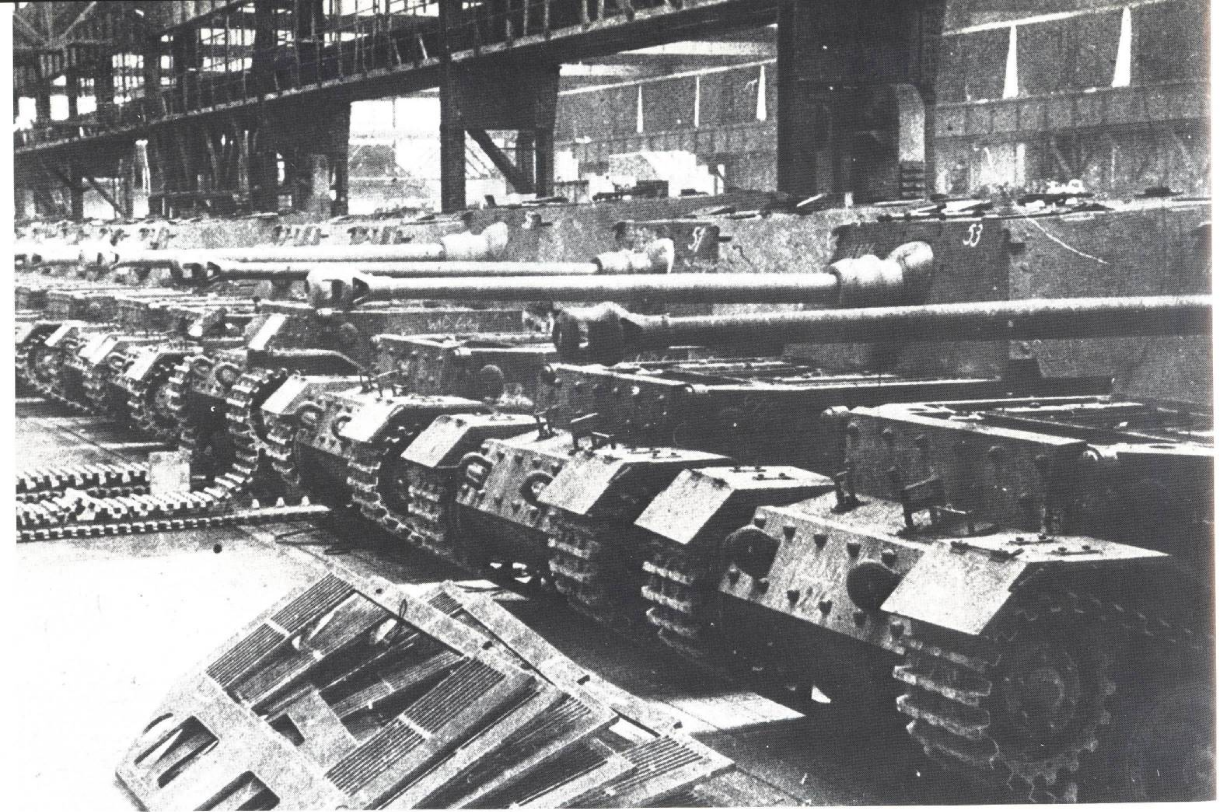
When in 1942 the decision was made in favor of the Henschel Tiger, the 90 Tiger (P) tanks already under construction were rebuilt as 8.8 cm Tiger (P) tank destroyers. This picture affords a view of the production building of the Nibelungen Works, where the completed vehicles are lined up ready for delivery.
